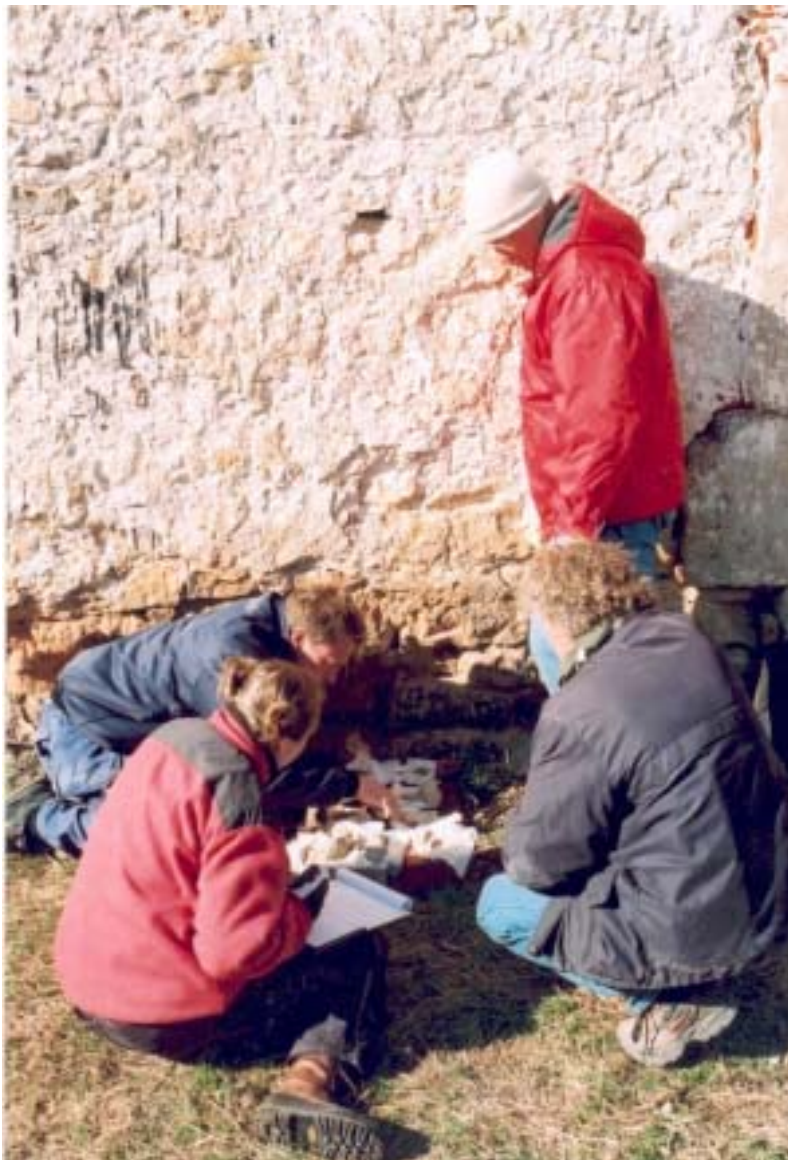
Acid testing of plaster samples
